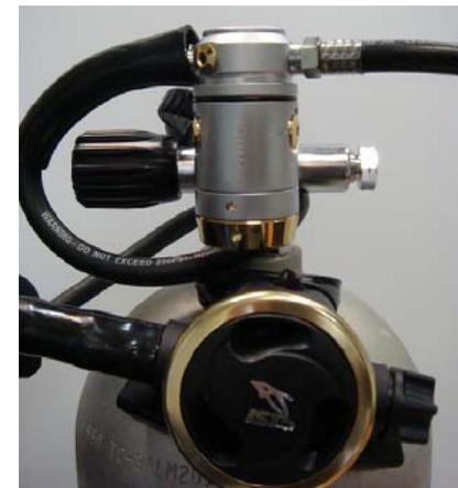
△ Only attach the hose to a regulator's low pressure port. Attaching to the high pressure port can cause the hose to burst, which may result in serious injury or death.
