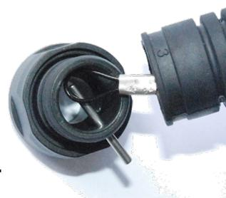
Make sure the adapter sleeve is in place and the hose is not pushed tight against it, or it will not spin freely. Secure the barbed end to the hose with a new cable ties.
