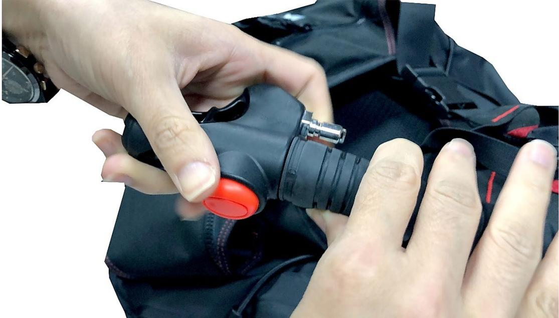
2-3. If there is a pull-dump wire connected, use a sharp cone to push and remove the pin on the inflator and disconnect the wire.
